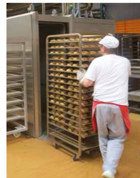
++ Vacuum cooling gives the range of bread rolls longer lasting crispness
